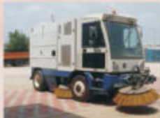
Self propelled with hydro-static drive
