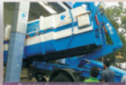
Portable Compactor lifting with Hook Loader
