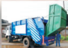
3.5M3 Bin being lifted into Garbage Compactor
